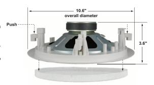
Installation: The 40AE has an integral mounting system that requires only a phillips screw driver to quickly flush mount the speaker into a 9.5" to 10" diameter hole. Before mounting the 40AE speaker, push the four mounting brackets to pop off the grill as shown in the diagram.
