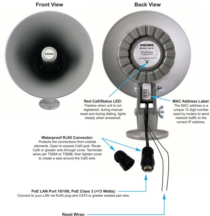
Open the waterproof RJ45 connector and remove black wires. Short wires during power up to reset security code or network parameters to factory
