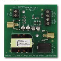
into a phone line, and converting a speaker level signal down to a line level signal.
