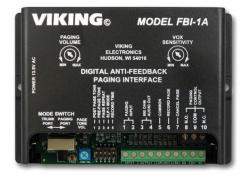
page length for faster processing. In addition, the **FBI-1A** can be programmed to provide pre-page and post-page alert tones.
