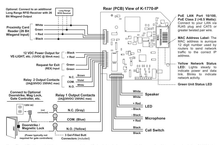
Note: The gel-filled (water-tight) butt connectors are designed for insulation displacement on 19-26 gauge wire with a maximum insulation of 0.082 inches.
