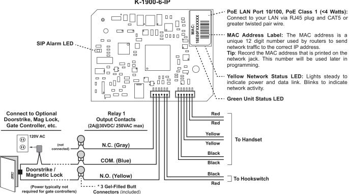
\*Note: The gel-filled (water-tight) butt connectors are designed for insulation displacement on 19-26 gauge wire with a maximum insulation of 0.082 inches.
