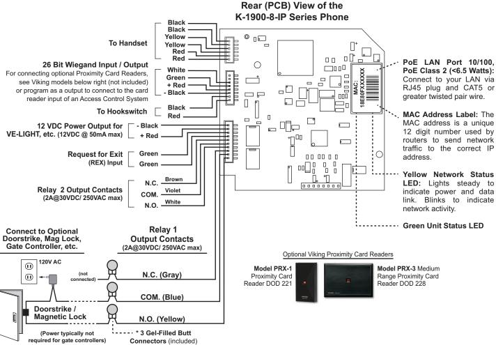
Note: The gel-filled (water-tight) butt connectors are designed for insulation displacement on 19-26 gauge wire with a maximum insulation of 0.082 inches.
