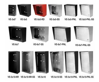
The **VE-PNL**'s are **VE-Series** backboxes with a blank aluminum panel. The user can customize the clear-coated aluminum panel to mount an **PRX-1** card reader, **PRX-2** keypad or switch. The kits come complete with box, gasket, panel and screws. Model numbers that end with "SS" are stainless steel version. **Note:** The use of magnets to mount the **VE-Series** enclosure to a metal surface can affect the operation of the enclosed product.
