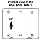
Mount the back panel to a wall, a single gang box or a 4" x 4" junction box with the arrow pointing up.
