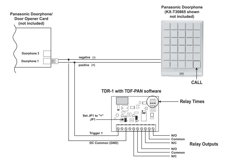
The TDR-1 detects when a user presses the "call" button on a Panasonic doorphone and provides a dry contact closure. This contact closure is adjustable from 1 to 60 seconds and can be used to activate a camera, a doorbell/chime or turn on lights. The TDR-1 requires special software model "TDF-PAN" for this application. Order the TDR-1 with TDF-PAN software installed. We will install and test the software for a nominal fee.
