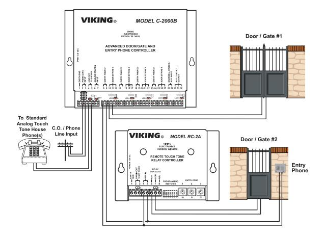
The C-2000B allows an entry phone to control one doorstrike relay, so a second entry phone is normally required to control two doors or gates. A Viking RC-2A can be added to allow a single entry phone to control a second door or gate. The keyless entry of the C-2000B operates the first door and the code set in the RC-2A operates the second.
