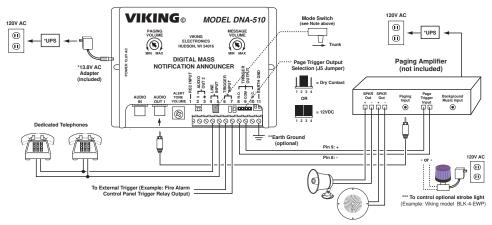
\* Caution: Uninterrupted Power Supply (UPS) recommended. UPS should have sufficient backup time to allow for emergency communication during a power outage. Maximum power consumption: DNA-510: 10 watts.
