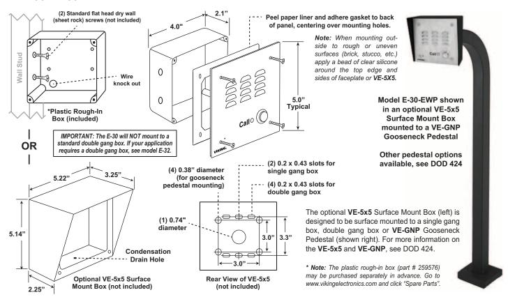
Caution: When warm air comes in contact with cold surfaces, such as outside walls and conduits, it causes condensation. To prevent condensation from accumulating inside the E-30/32 always bring conduit into the bottom of the unit. If this is not possible, drill a 1/4" diameter hole in the bottom of the gray plastic box.
