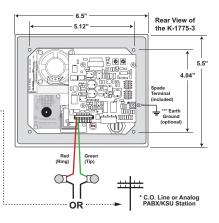
\*\* Note: The gel-filled (water-tight) butt connectors are designed for insulation displacement on 19-26 gauge wire with a maximum insulation of 0.082 inches. Cut off stripped wire ends prior to terminating.
