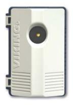
This auxiliary electronic ringer operates on any analog line that provides a minimum of 40 volts 20-30 Hz AC ring voltage. Nominal 3 KHz warble provides adequate volume for business offices. The **LPR-1** can be connected via screw terminals or modular RJ-11 jack. A volume control and a 7 foot modular cord are provided. No power supply is required.
