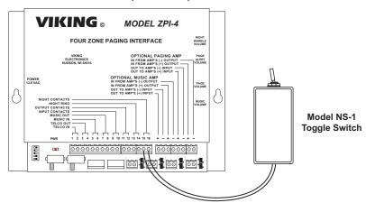
For remote mounting, remove the base from the **NS-1** and cut off the connection wires inside the case. Now use the provided quick connectors to make connection to an extension cable. Replace the base. Peel off the protective liner from the foam tape on the bottom of the **NS-1** and firmly press it onto the mounting surface. Connect the other end of the extension cable to the controlled equipment.
