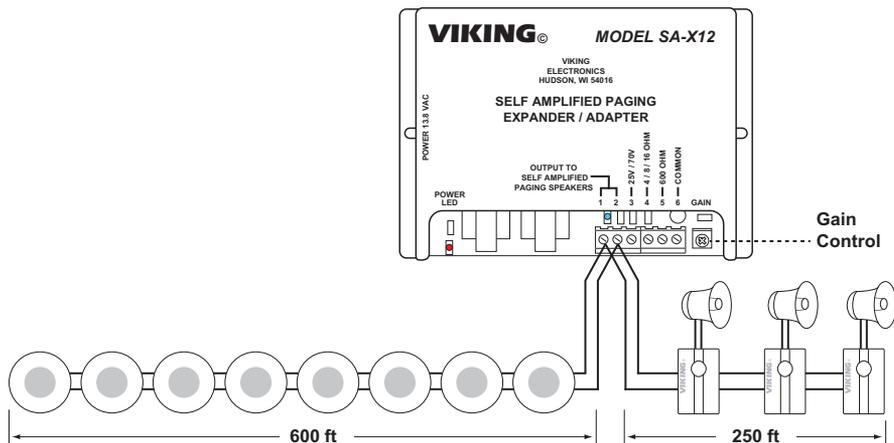
**Example:** Eight (8) **SA-1S** speakers on a 600 ft long wire run. Use at minimum #18 AWG copper wire pair as recommended in the Wire Gauge Chart on page 2.
