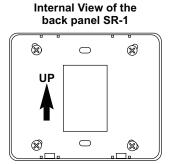
Mount the back panel to a wall, a single gang box or a 4" x 4" junction box with the arrow pointing up.
