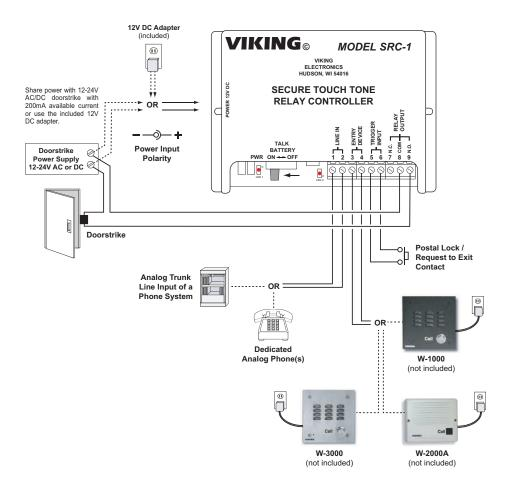
B. Line Powered Entry Phone to CO Line or Analog PABX/KSU Station (Talk Battery Provided by Line In)
