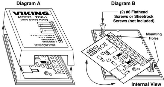
**Important:** Make sure the screw heads are fully driven into the base to avoid shorting the circuit board leads.
