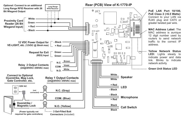
**Note:** The gel-filled (water-tight) butt connectors are designed for insulation displacement on 19-26 gauge wire with a maximum insulation of 0.082 inches. Cut off stripped wire ends before terminating.
