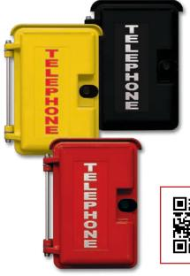
The VE-9x12 series of outdoor enclosures provide the ultimate in weather protection for your Viking product or other device. The VE-9x12 enclosures are constructed of durable UV stable polycarbonate / ABS composite to provide years of outdoor service. The heavy-duty doors are labeled "Telephone" and have a gasket seal to keep out even the harshest weather. The VE-9x12 allows you to choose from three panels that allow mounting many different Viking products.
