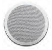
The Viking model **40-IP** Speaker enables SIP endpoint paging and also allows for standard paging and background music via multicast. The speaker easily connects with a single CAT5/6 cable from your PoE switch. Its shallow depth allows the speaker to be conveniently mounted in a standard 2" x 4" stud wall or ceiling. Line-level audio output connections are provided for connecting to an external amplifier. A built-in 6 Watt class D amplifier with speaker output connections is also provided.
