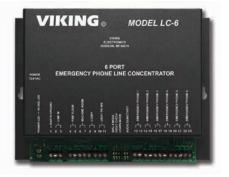
All telephone line inbound calls are answered by the LC-6. A touch tone command will route the call to any of the phone ports. If no command is detected within 4 seconds, the call will be routed to the last emergency phone that was used. This allows emergency personnel to easily call back to the same phone.
